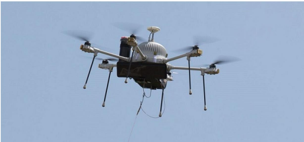
This aerial small cell was manufactured by Airspan, a leading vendor of LTE small cells and backhaul technologies. At the heart of the small cell are two powerful chipsets – one from Qualcomm Technologies (Qualcomm® FSM™) for the base station portion of the small cell, and one from GCT Semiconductor for wireless backhaul. GCT's LTE Advanced GDM7243Q chip enables faster LTE speed and improved coverage with 4Rx antenna technology and 2Tx diversity technology.
